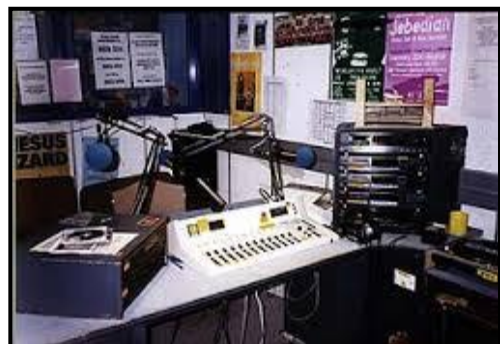
Microphones connected to a broadcast console and CD and tape players. Image from members.tripod.com
